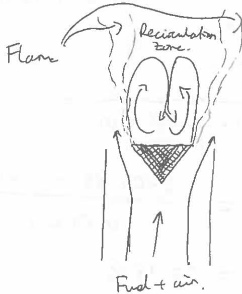
The bluff body creates a low-velocity region of recirculating flow. This region contains hot combustion products as they are transported from the flame to the anchoring point to ignite incoming reactants and therefore, the recirculation zone is a constant ignition source.
