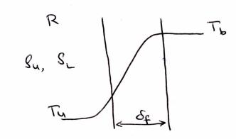
energy Generated  $\approx$  Conducted  $\dot{w}_{cp}(T_{b}-T_{u}) A \delta_{f} \approx \lambda A \frac{(T_{b}-T_{u})}{\delta_{f}}$ =)  $\left( \delta_{f}^{2} \approx \frac{\lambda}{\dot{w}_{cp}} \right)$
