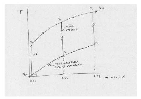
(d) The maximum pressure is reached when the reaction is complete. Under those conditions, x = 1, and the final pressure is reached, which can be extracted from the transcendental equation below:
