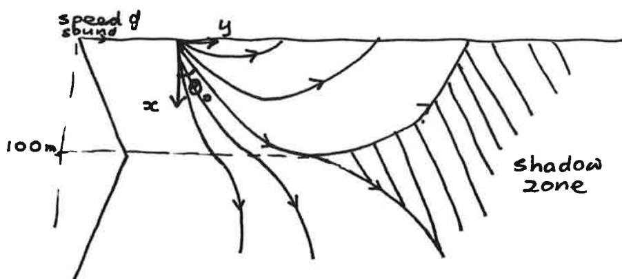
b) (i) The ray that forms the boundary of the shadow zone is horizontal at  $x = 100m$ . Hence the angle  $\theta_0$  between the vertical axis and the ray at the surface is given by
