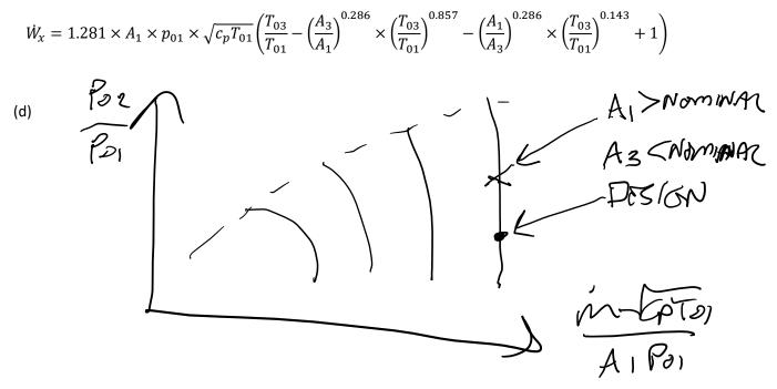
Change schedule of variable guide vanes. To implement this the first few stages of the compressor would have to have variable guide vanes. This involves implementing a variable guide vane mechanism and scheduling the vanes correctly at each operating point.
