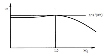
For supersonic flow the turbine passage is a convergent-divergent nozzle. For the divergent section the exit angle must reduce. The limiting exit Mach number occurs when the axial Mach number is one. At this point pressure waves cannot travel upstream and this therefore the exit Mach number cannot rise any further.
