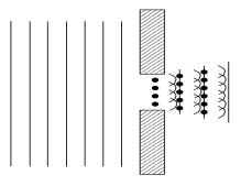
Assumptions: Plane wave coherent (laser) illumination of the aperture. Only consider forward propagating waves. Aperture is larger than wavelength x2.
