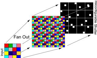
Optical fan-out can be done by the illumination of a  $k \times k$  spot CGH or Damman grating to replicate the source inputs. The use of the CGH to replicate the inputs comes from the CGH property that the spots in the replay field are the FT of input illumination. In past examples this has been Gaussian, but it could equally be an input structure or an array of input sources.
