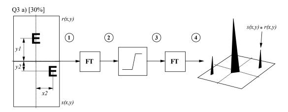
Plane 1 is the input plane with reference and object place side by side. This is usually done optically using a liquid crystal spatial light modulator.
