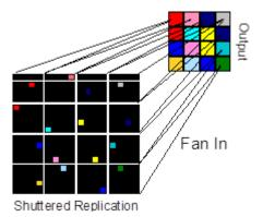
The problem with this process is that the output array is formed via the fan-in optics which only send one replicated array per output channel. In this system multiple outputs can be switched to by opening the same shutter is two different replications. If the output array contains more that n fibres, then the fan-in process could be adapted to accept multiple combinations of inputs, forms a limited broadcast capability.
