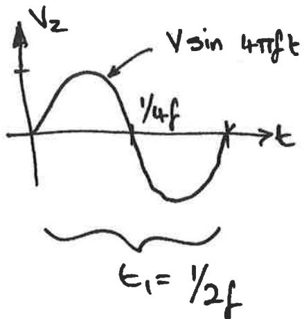
If we assume the waveform is a sine wave and integrate a  $V_2$  cycle,
