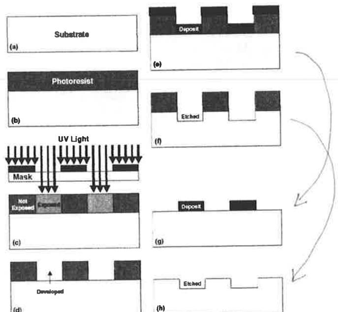
Then, either a deposition process eg. Chemical Vapour Deposition (CVD), evaporation or sputtering deposits a metal, ceramic or Si layer on the wafer (e) or the underlying substrate / layer is etched (f). The photoresist layer is then usually removed by dissolving in solvent (eg. acetone) or plasma etched to leave the processed substrate (g) or (h).
