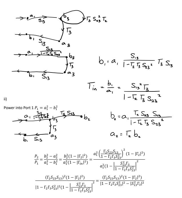
This was generally answered quite well. Common mistakes included an assumption that B=C in the transmission matrix due to the reciprocal network, but this doesn't work due to the current definitions. In b(ii) most did not realise that the  $a_2$  and  $b_1$  terms need subtracting to get the power into the load (and not reflected) and the power into the network (and not reflected).
