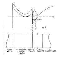
The electrons in the GaAs are in a triangular well, and are confined to a sheet parallel to the surface, just a few nm thick. This is known as a two-dimensional electron gas.
