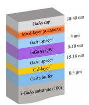
A semiconductor heterostructure is created when layers of different semiconductors (typically with different bandgaps) are grown sequentially. A standard growth technique is Molecular Beam Epitaxy that allows the deposition of single monolayers of semiconductors in a controlled, high vacuum environment.
