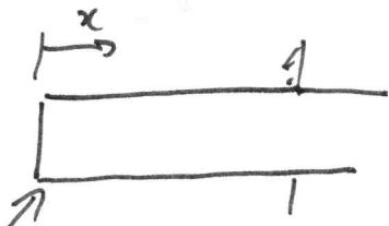
At failure this point starts to slip
