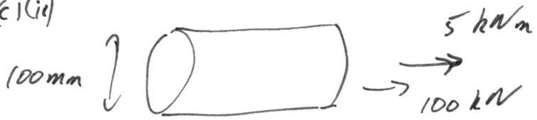
$$F = N_x \pi D \Rightarrow N_x = \frac{100 \text{ kN}}{\pi \cdot 100 \text{ mm}} = \frac{1}{\pi} \frac{\text{MN}}{\text{m}}$$
