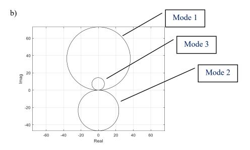
The response is measured on the top floor. Modes 1 and 3 therefore involve responses that are in-phase with the excitation, hence circles on the positive imaginary axis. Mode 2 involves an out-of-phase response, hence a circle on the negative imaginary axis.
