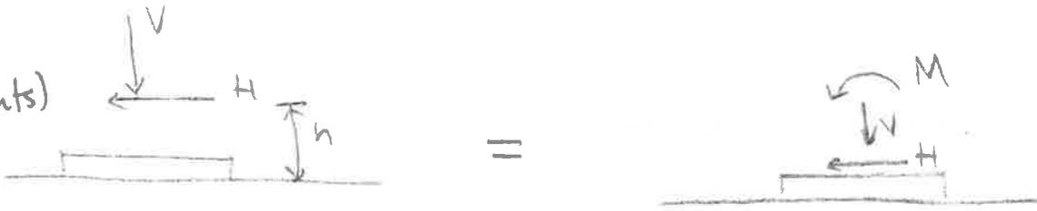
When the horizontal load is applied above the plane of the foundation it generates a moment.
