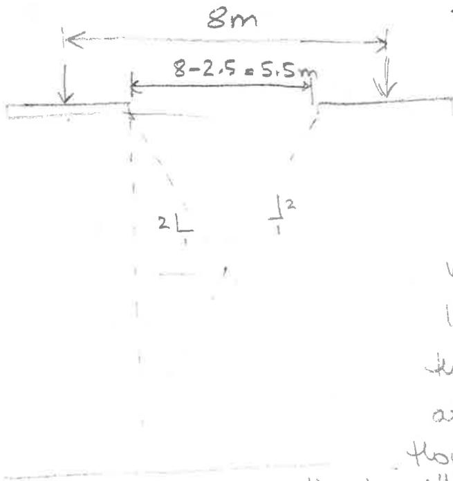
Not very worried about load interaction at depth. With a rough estimate of load spreading at a 2:1 slope the interaction would start at 5.5m between two footings. However interaction below the edge of the foundation would occur at 11m depth.
