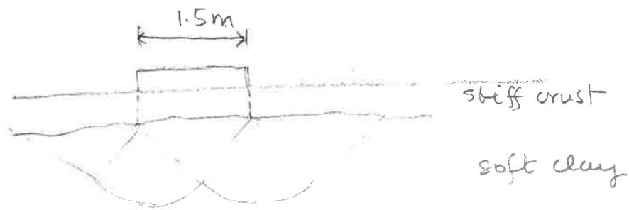
The stiff crust would likely be punctured as the clay settles. Therefore, we could assume that the failure occurs through the clay and the stiff crust would act as an overburden.
