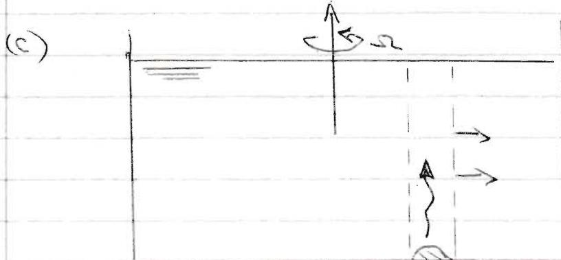
Slowly moving object emits low-frequency waves. These travel upward with a group velocity of  $|c_g| = 2 \pi L$  where  $L$  is the size of the object. The waves carry the information that the object is moving.
