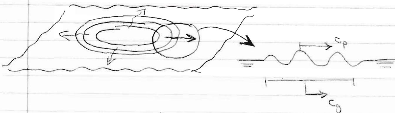
The overall wave packet travels at  $c_g$  which is ~~one~~ half the speed of the wave crests, which travel at  $c_p$ .
