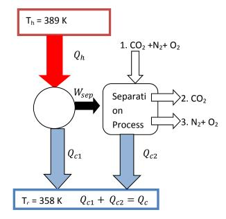
The minimum work to separate gases can be calculated from the first and second law applied to a control volume, just around the separation process,
