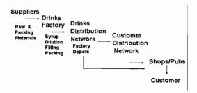
The supply chain must also be monitored in order to affect control over the full manufacturing cycle. In the case of a soft drinks manufacturer the supply chain can be described as follows.
