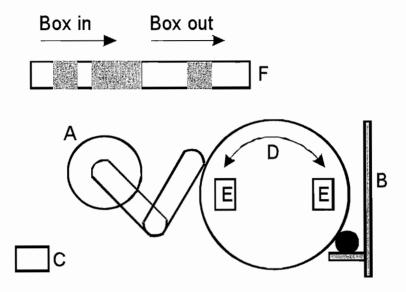
b) The fixture used for the automated assembly would be duplicated on either side of the rotary table. Its primary function is to locate components that need to be assembled and hold them in place during the fastening process.
