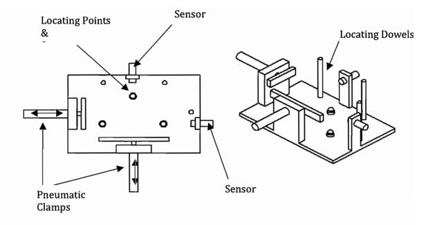
c) The most suitable types of sensors for this application would be none contact, such as optical diffused, or capacitive. These types of sensors work well with plastic components and can be purchased in a thread barrel type package that allows them to be easily positioned in the fixture for optimal operation. Due to their non-contact operation they have a much better operating life than typical contact devices.
