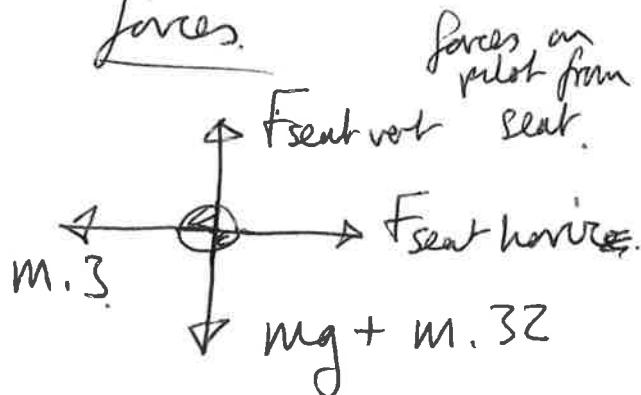
$$\begin{aligned} F_{\text{seat vert}} &= mg + m.z \\ &= 80(9.81 + 32) \\ &= 3344.8 \text{ N} \end{aligned}$$
