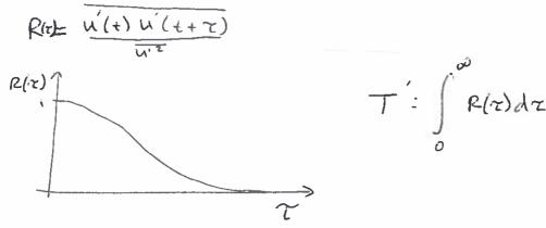
The hot wire must be able to resolve the velocity fluctuation across the smallest eddy as it is being convected past the probe by the mean velocity U, hence the fastest frequency must be  $V/\eta_{K}$ . The integral timescale T' is related to the eddy turnover time  $T=k/\varepsilon$  (or  $L/k^{1/2}$ ) by T'=L/U.
