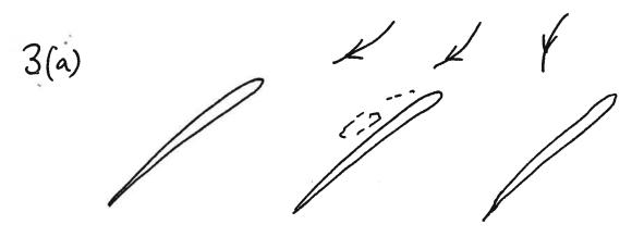
A local flow perturbation causes one blade passage to exhibit separation (or other rise in blockage). Flow is divorted around this blocked passage increasing incidence for blades to the left, which then separate, and reducing it for blades to the right which, if separated, then recover. The pattern grows to cover a number of passages - a cell - which propagates around annulus.
