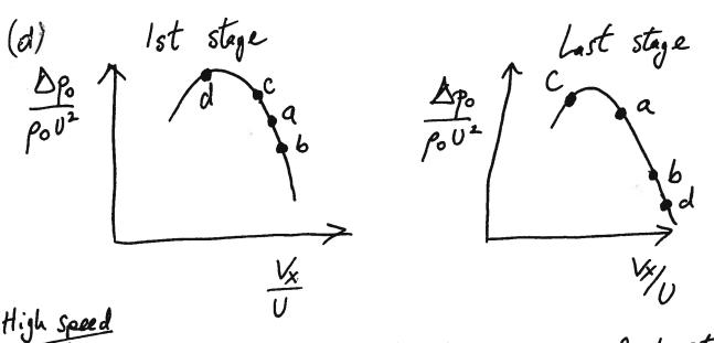
As miss flow increases density rise aarss first stage is less than design => Vx into second stage > Vxdosign => less density rise. Process same through machine, so Vx 1 point to for last stage near chake. Opposite effect for point c - last stage sees much lower Vx
