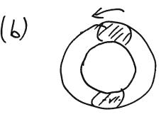
High hub-to-tip ratio likely to be full span stall
