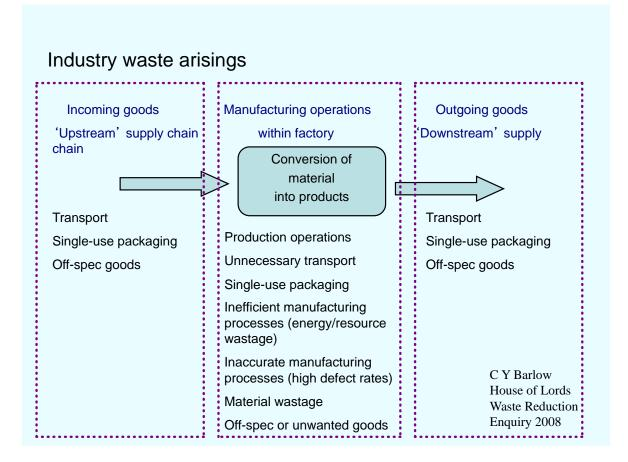
Environmental impact: Material wastage most important, then energy for factory operations and space heating. Impact can be assessed by performing a full environmental audit of the factory and its operations; indications of likely rankings can be obtained from McKinsey Abatement curves which are discussed further in (b).
