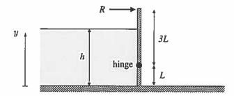
(a) The force on the gate is the integral of the hydrostatic pressure on its surface. On the air side  $p = p_a$ , and on the water side  $p = p_a + \rho g(h - y)$ , so the resultant is
