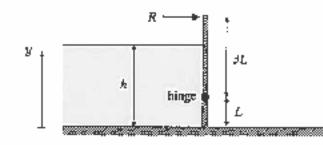
(a) The force on the gate is the integral of the hydrostatic pressure on its surface. On the air side  $p = p_a$ , and on the water side  $p = p_a + pg(h + y)$ , so the resultant is
