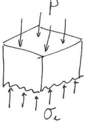
Using the usual convertion that stresses are the if tensile:  $-4Lt O_{L} = P.L^{2}$  $:: O_L = -\frac{PL}{4t}$
