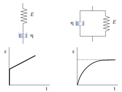
Spring and dashpot in series: The first part is the instantaneous elastic response while the second part is the viscous retarded response.
