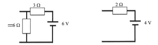
(The open circuit voltage from the circuit on the left =  $6 \times \frac{6}{6+3} = 4 V$
