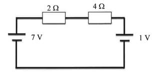
The current flowing in the circuit is the total potential difference divided by the total resistance around the circuit
