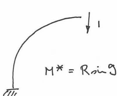
$$\begin{aligned} v &= \int_0^{\pi/2} (R \sin g) \left( -\frac{WR}{\pi} + \frac{W}{2}R \sin g \right) \frac{R dg}{EI} \\ &= -\frac{WR^3}{\pi EI} + \frac{WR^3}{2EI} \int_0^{\pi/2} \frac{1 - \cos g}{2} dg \\ &= \frac{WR^3}{EI} \left[ \frac{\pi}{8} - \frac{1}{\pi} \right] \end{aligned}$$
