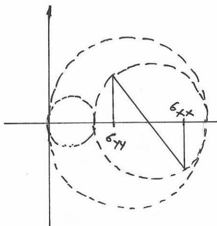
$$\begin{aligned} \frac{\sigma_{xx} + \sigma_{yy}}{2} + R &= Y \\ \frac{3P}{4} + \sqrt{q^2 + P^2/16} &= 1 \\ \rightarrow \boxed{q^2 - \frac{P^2}{4} + \frac{3P}{2} = 1} \end{aligned}$$
