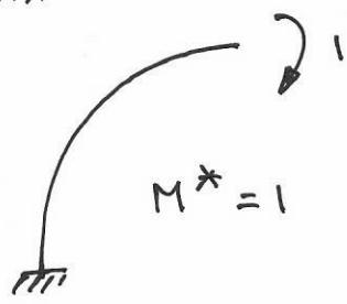
$$\begin{aligned} g &= \int_0^{\pi/2} \frac{MM^*}{EI} R dg = \frac{R}{EI} \int_0^{\pi/2} (Q + PR \sin g) dg \\ &= \frac{R}{EI} \left[ Q \frac{\pi}{2} + PR(-\cos g) \right]_0^{\pi/2} = \frac{R}{EI} \left[ Q \frac{\pi}{2} + PR \right] \end{aligned}$$
