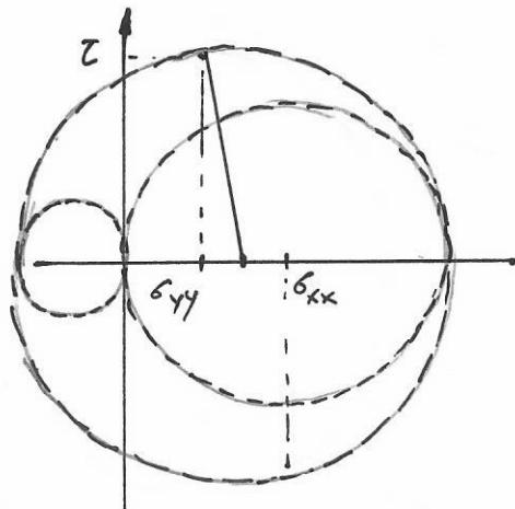
$$\begin{aligned} R &= \sqrt{\tau^2 + \left(\frac{\sigma_{xx} - \sigma_{yy}}{2}\right)^2} \\ &= Y \sqrt{q^2 + \frac{(P/2)^2}{4}} = Y \sqrt{q^2 + P^2/16} \\ Y/2 &= Y \sqrt{q^2 + P^2/16} \\ \boxed{16q^2 + P^2 = 4} \end{aligned}$$
