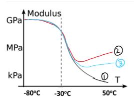
Curve-1: No crosslinking, polymer chains flow above Tg and thus loss of elastic modulus. Curve-2 and Curve-3 are associated with a crosslinked elastomer, where the number of monomers between crosslinking points increases from Curve-2 to Curve-3. The form of the curves reflect that for an elastomer above the glass transition temperature, the elastic modulus (*E*) scales with  $T/n_c$ , where  $n_c$  is the number of monomers between cross-links.
