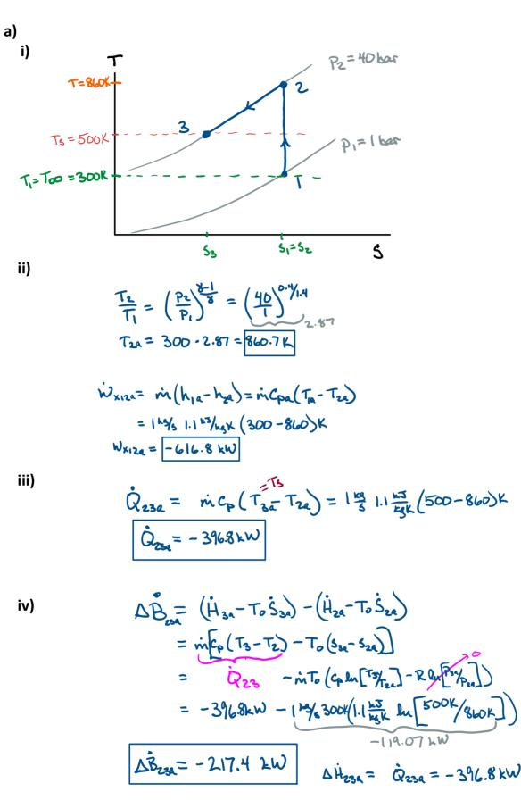
**Discussion:** The change in available power represents the maximum amount of work that could have been produced in a Carnot heat engine exchanging heat with a finite temperature,  $T_{\infty}$ . The change in availability is less than the change in enthalpy as only a fraction (Carnot efficiency) is available for work. The question solely pertains to the changes in enthalpy and availability of the air and not the thermal storage.
