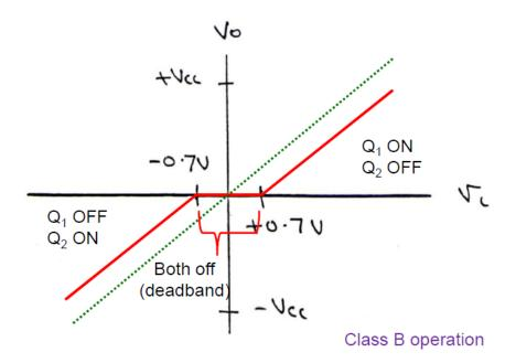
This creates extra harmonics in the signal at the output causing distortions.
