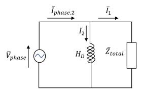
$I_{phase,2} = I_1 + I_2$ , where  $I_1 = I_{phase}$ , i.e., the phase current before correcting the power factor.
