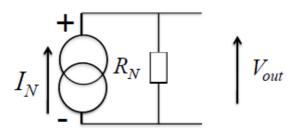
Here,  $I_N$  is the short circuit current of the original circuit.  $R_N$  = open circuit voltage/short circuit current.
