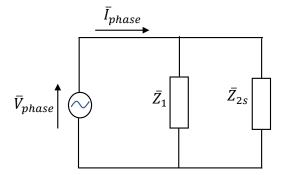
For the star-connected supply:  $V_{phase} = \frac{415}{\sqrt{(3)}} = 240 \text{ V.}$ For the star-connected load:  $\bar{Z}_1 = R || \frac{1}{j\omega C} = \frac{R}{1+j\omega C} = \frac{400}{1+j2\pi \times 50 \times 10 \times 10^{-6} \times 400}$ = 155.19 - j194.91  $\Omega$
