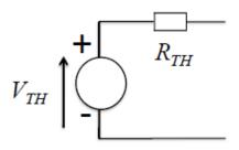
Here,  $V_{TH}$  is the open circuit voltage of the original circuit ( $V_{out}$ ).  $R_{TH}$  = resistance measured between output terminals of original circuit.
