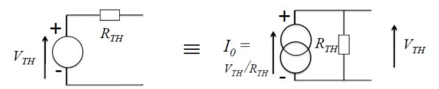
These equivalents can then be used to simplify more complex circuits and circuit elements.
