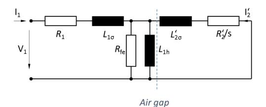
$\begin{array}{l} R_1: \mbox{ copper resistance in stator} \\ L_1: \mbox{ stator stray inductance/reactance} \\ R_{fe} \mbox{ or } R_i: \mbox{ equivalent iron-loss resistance} \\ L_{1m}: \mbox{ magn. reactance} \end{array}$
