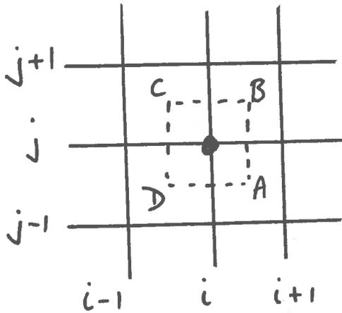
On AB  $\frac{\partial \phi}{\partial n} = \frac{\phi_{i+1,j} - \phi_{i,j}}{\Delta x} \Rightarrow \int_{AB} \frac{\partial \phi}{\partial n} dS = \frac{\phi_{i+1,j} - \phi_{i,j}}{\Delta x} \Delta y$
