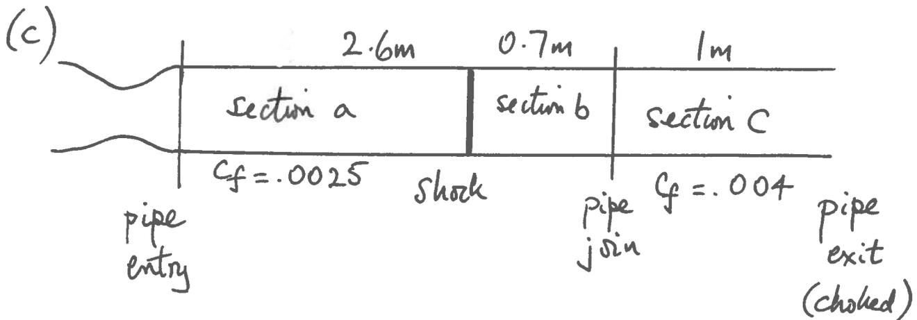
In section c  $\frac{4 C_f L}{D} = \frac{4 \times 0.004 \times 1}{0.2} = 0.08$
