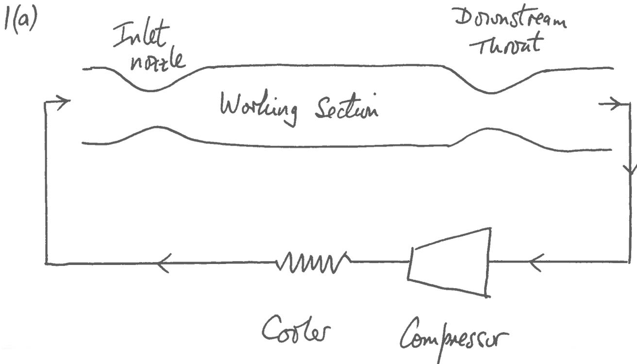
Isentropic operation is not possible due to viscous effects and the need to decelerate the flow which will involve a shock in a fixed geometry tunnel.
