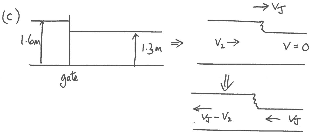
$$V_J(V_J - V_2) = \frac{1}{2} g(h_1 + h_2) \text{ and } \frac{V_J^2}{gh_1} = \frac{1}{2} \frac{h_2}{h_1} \left( \frac{h_2}{h_1} + 1 \right)$$
