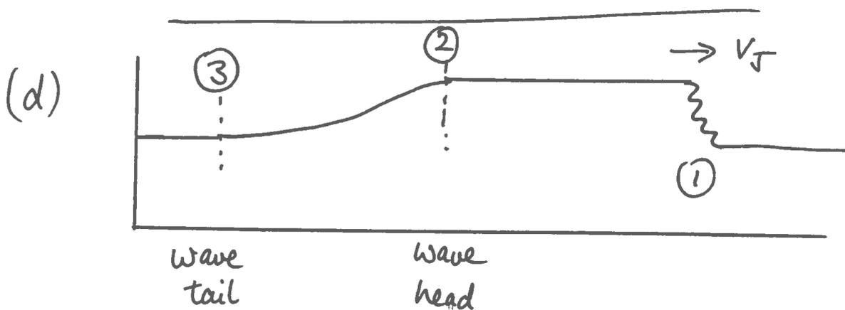
Right running waves  $V_3 - 2C_3 = V_2 - 2C_2$
