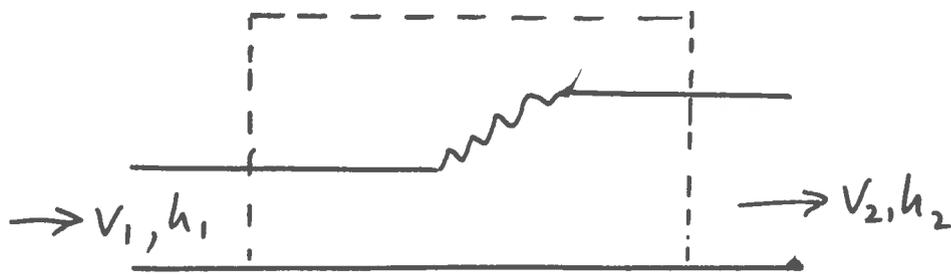
Continuity:  $h_1 V_1 = h_2 V_2$
