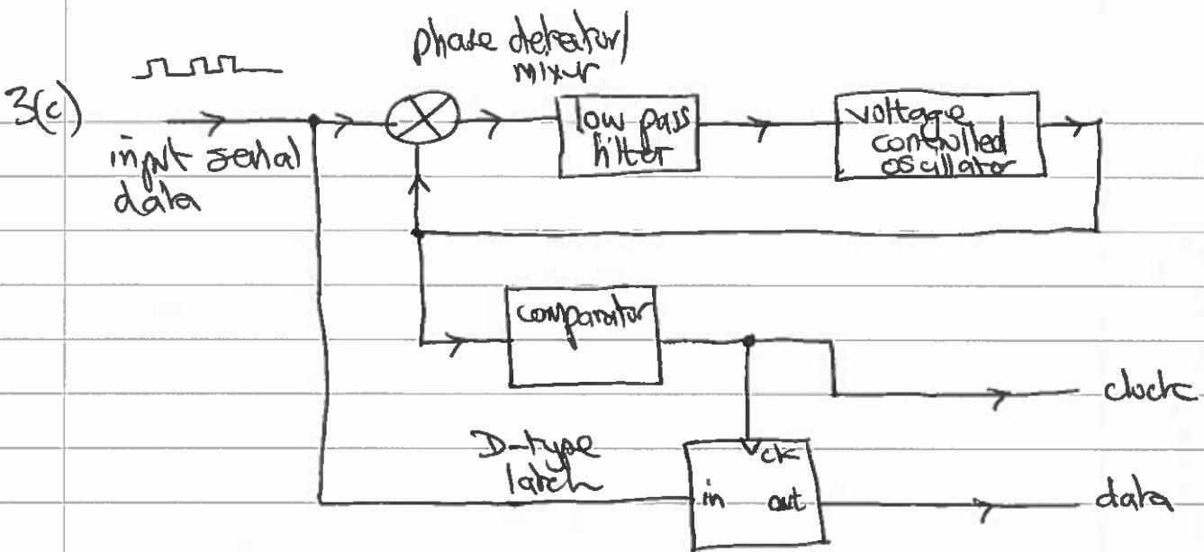
A comparator is included if the VCO has an analogue output - to synchronize the clock and data streams of bits a D-type latch is included.
