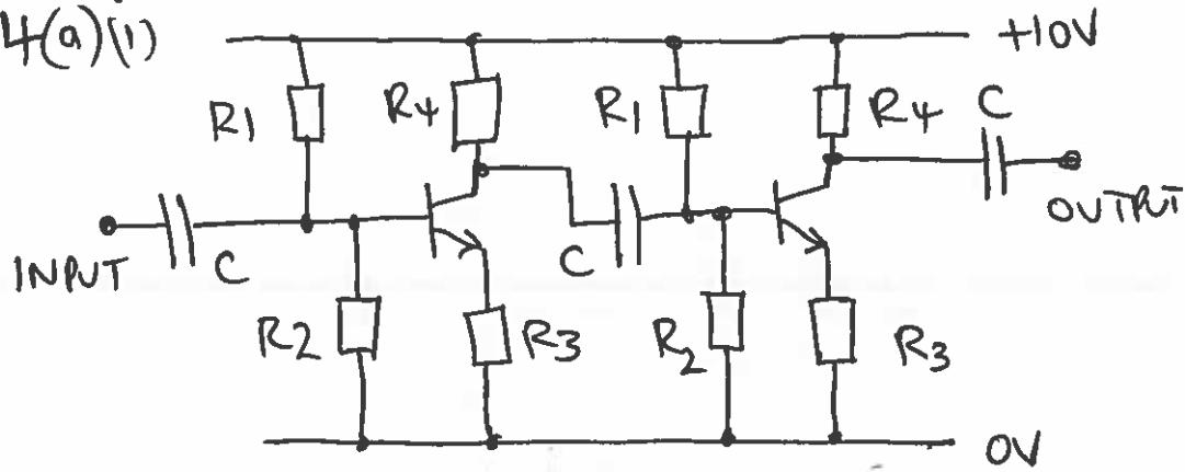
$R_1, R_2$  : base bias resistors, set base-emitter voltage at  $\approx 0.6V$  and  $V_c$  at  $\approx \frac{1}{2}$  supply
