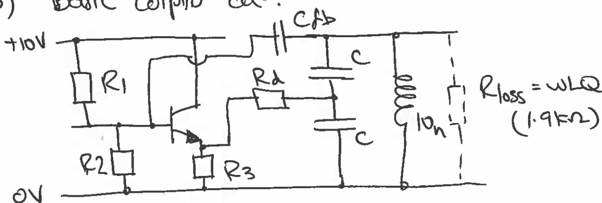
$R_1$  and  $R_2$  set base @  $\sim 5.6V$  and are  $\sim$  few kΩ each (to match loss resistor).  $\therefore R_1 = 2k7$ ,  $R_2 = 3k3$
