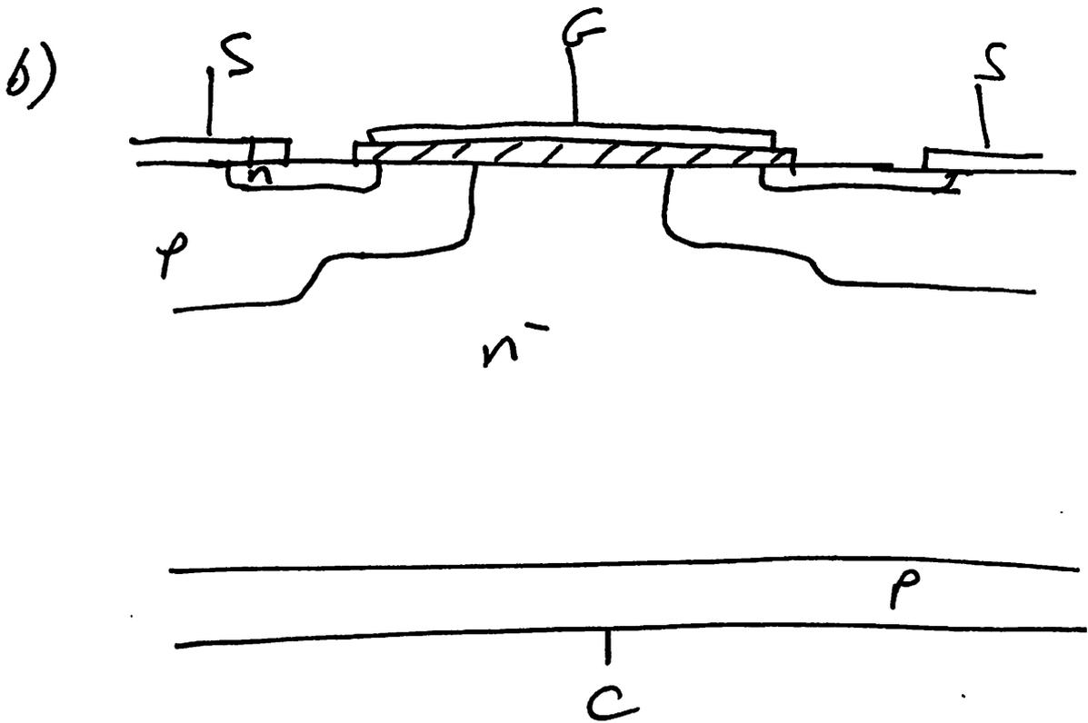
The bipolar is pnp so electrons are needed. These are provided by the MOS Channel formed in the p at the top
