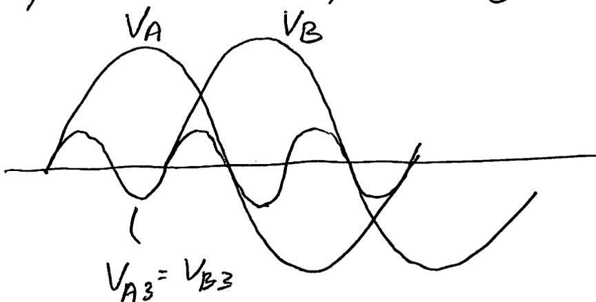
Since any output is across any two legs eg.  $V_A - V_B = V_{AB}$  then the third harmonics have no contribution to  $V_{AB}$  as they cancel.
