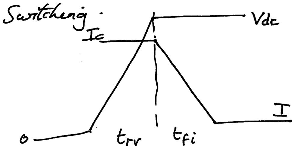
$$\begin{aligned} \text{Energy} &= I_c \cdot V_{dc} \cdot \frac{t_{rr}}{2} + V_{dc} \cdot I_c \cdot \frac{t_{fi}}{2} \\ &= \frac{I_c V_{dc}}{2} (t_{rr} + t_{fi}) \end{aligned}$$
