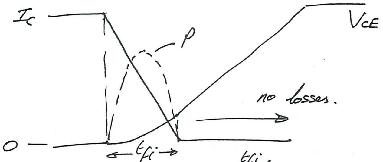
$$V_{CE} = \frac{1}{C} \int i_c dt = \frac{1}{C} \int_0^{t_{fi}} \frac{I_c}{t_{fi}} dt$$
