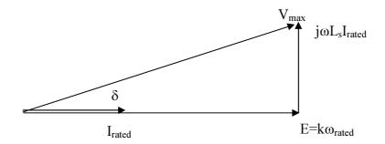
Noting that  $V_{max}=415/\sqrt{3}$ ,  $I_{rated}=40$  A, Ls=8 mH and  $\omega=p\omega_{rated}$  where p is the number of pole-pairs which is 2:
