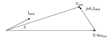
The torque angle may be found from  $T = 3kI\sin\beta$  giving  $60 = 3 \times 0.8 \times 50 \times \sin\beta$  and so  $\beta = 30^{\circ}$ .
