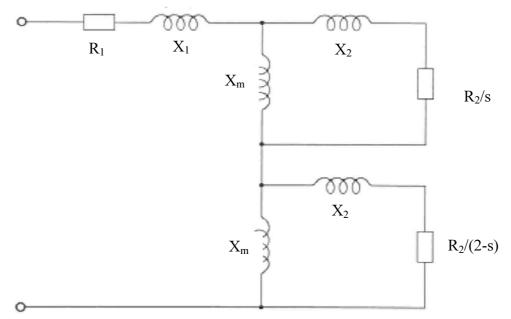
The torque-speed curve is obtained by superimposing the torque-speed curves of two three-phase induction motors, one forwards rotating, the other backwards rotating, but both producing torque in their directions of rotation.
