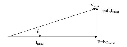
Noting that  $V_{max}=415/\sqrt{3}$ ,  $I_{rated}=50$  A,  $L_s=4$  mH and  $\omega=p\omega_{rated}$  where p is the number of pole-pairs which is 3:
