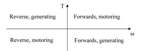
An application where 4 quadrant drive control is desirable is the electric vehicle. Clearly the vehicle needs to be able to be driven both forwards and backwards. It is desirable if the drive can generate power back to the battery when it is braked, as this improves efficiency. Regenerative braking requires 4 quadrant control if it is to be used to brake the car when it is travelling forwards or backwards.
