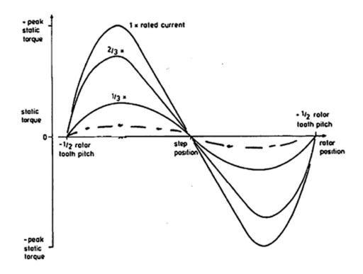
(iii) Position error is defined as the angular deviation away from the full-step equilibrium position caused by a static load torque. Modelling the motor torque as
