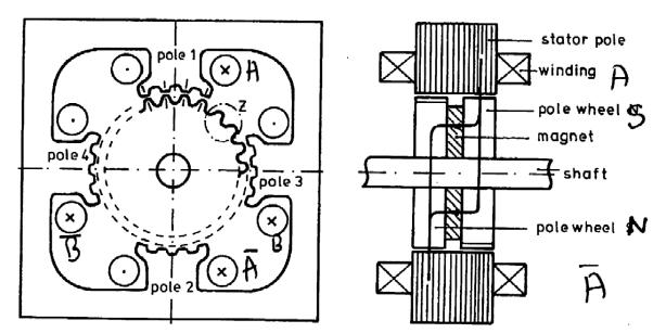
Rotor: soft magnetic material with 50 equally-spaced teeth, with an axially-magnetised PM sandwiched between. Rotor wheels offset from each other by exactly 1/2 tooth pitch. Stator: coils wound on each pole, coils making up each phase connected in series.
