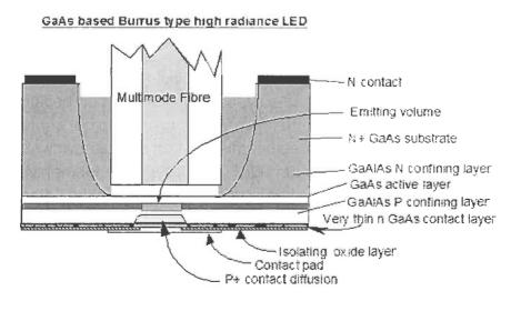
The Burrus diode has much of the substrate etched away: this allows high coupling into a multimode fibre. Sometimes a spherical micro-lens is introduced as well. In addition, the heat generation is close to the p surface which can be bonded directly to a heatsink and the contact metal also reflects some light back upwards into the fibre. Similar devices are made using the InP/GainAsP materials system at longer wavelengths.
