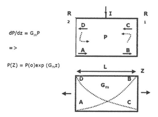
The photon lifetime of the laser cavity can be readily determined by considering the amplification of laser light as it propagates along the laser cavity. Assume that stimulated emission encounters a gain per unit length (due to stimulated amplification), G, and a loss per unit length due to scattering, G, as it passes along the laser. The gain G in practice creates extra photons to compensate for those photons lost as the signal travels over a distance of unit length.
