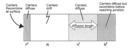
The overall time response can be broken down into two separate regions of operation, the response of the depletion region and the response of the diffusion region. These responses are shown schematically below.
