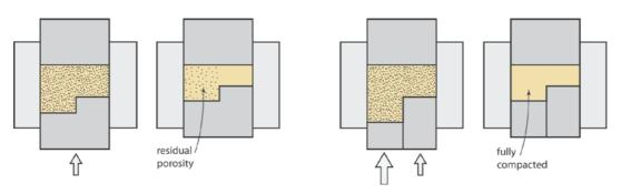
(b) Assume that there is no flow of material between the two parts of the die, so compaction occurs uniaxially in each half, i.e. the volume of solid is separately conserved in each half, and the same vertical strain is applied.
