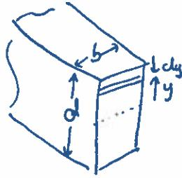
$$\underline{\text{Tension}} \quad T = \int_{-d/2}^{d/2} \sigma_{xx} \cdot b \cdot dy$$
