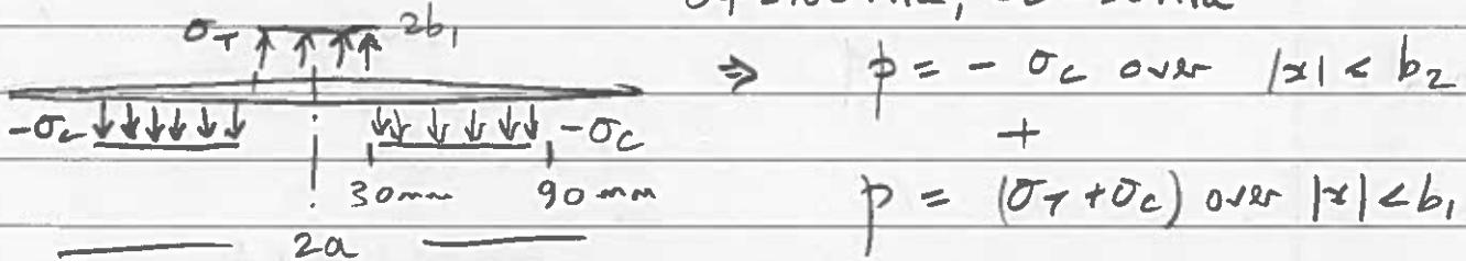
$$\text{So } K = 2(\sigma_T + \sigma_C) \sqrt{\frac{a}{\pi}} \sin^{-1}\left(\frac{b_1}{a}\right) - 2\sigma_C \sqrt{\frac{a}{\pi}} \sin^{-1}\left(\frac{b_2}{a}\right)$$
