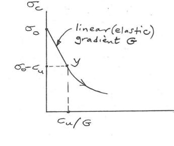
Clay yields at y,  $\sigma_c = \sigma_o - c_u$  $\sigma_c = 500 - 175 = 325 \, kN/m^2$
