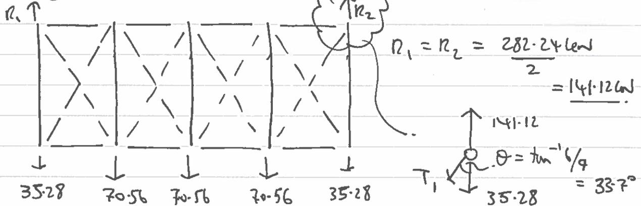
$$\begin{aligned} \therefore \text{ TENSION IN WOOD MEMBER } T_1 &= \frac{(141.12 - 35.28)}{\cos 33.7} \\ &= 127.2 \text{ kN} \end{aligned}$$
