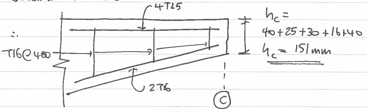
$h_A$  IS LIMITED BY SHEAR CRITERIA REINFORCEMENT AT A AND BY MINIMUM DEPTH OF BEAM FOR BENDING AT D.
