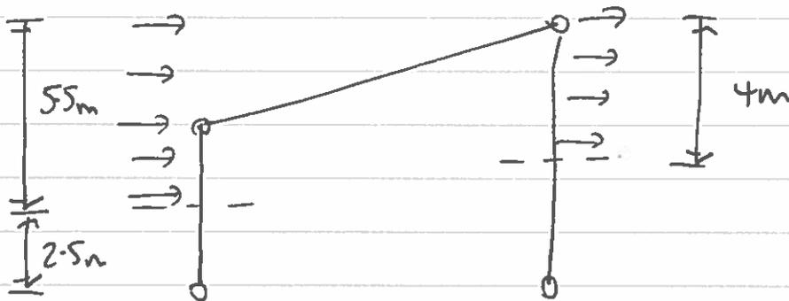
$$\begin{aligned} \text{LATERAL LOAD } P \text{ PER FRAME} &= \left[ (1.2 \text{ kN/m}^2) \times 5.5 \text{ m} \times 6 \text{ m} \right. \\ &\quad \left. + 0.8 \text{ kN/m}^2 \times 4 \text{ m} \times 6 \text{ m} \right] \times 1.2 \\ &= 70.56 \text{ kN} \end{aligned}$$
