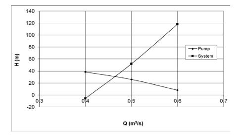
From the diagram: Q = 0.465 m<sup>3</sup>/s = 465 l/s, efficiency = 58%  $P_p = \rho g Q_p H_p / \eta = 1000 \times 9.81 \times 0.465 \times 32/0.58 = 251.67$  kW
