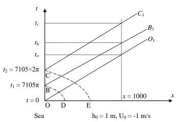
The first high tide occurs at the mouth at  $t_1 = 7105\pi = 22309.7$  s, with  $h_1 = 7$  m. Along –ve line BD
