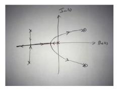
(ii) For what range of k are all the poles of the closed-loop system real valued? [20%] Need k between the values for the two breakawaypoints, ie k = 1/|G(s)| for s = -2 and -5.9, ie 0.46 < k < 0.74.
