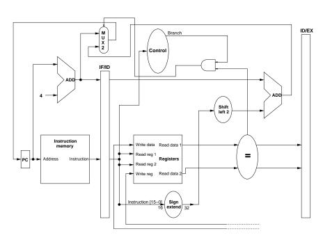
In the modified datapath, the branch target calculation is moved from the EX stage to the ID stage. The registers are also compared at the ID stage. Only one subsequent instruction
