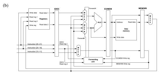
The forwarding unit compares the registers which have just been read ("read reg 1" and "read reg 2") with any registers about to be written by the two downstream instructions. If they are the same, it sets MUXA and/or MUXB to ignore the value read from the register file and instead use the appropriate forwarded value.
