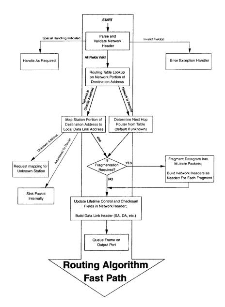
IoT - advantage of the fast path is that it will process data with low latency, hence any applications such as voice and video will work efficiently. There will be some cost in terms of complexity as the of the processing makes each node complex.
