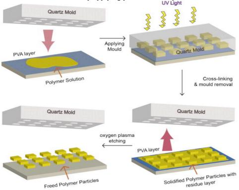
*Step-Flash Imprint Lithography (S-FIL).* A quartz mold with cavities of predesigned shapes is pressed against a photo-crosslinkable monomer solution on top of a silica wafer. A PVA layer is put beneath the polymer solution for the release of imprinted particles. The monomers are crosslinked by applying UV light. Residual layer from the crosslinking reaction is removed by oxygen plasma etching and particles are freed by dissolving away the PVA layer.
