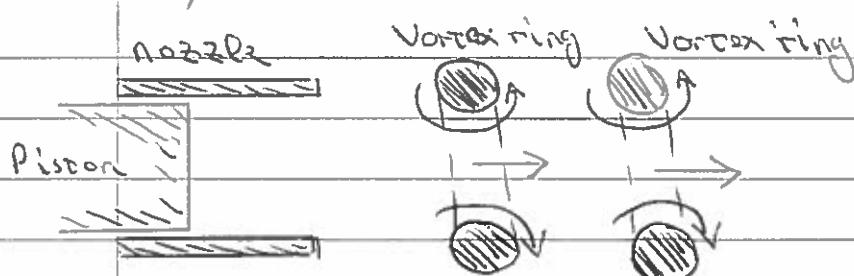
Create a pair of vortex rings (co-axial) using a piston and nozzle.
