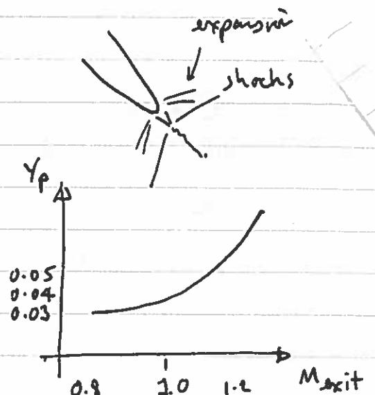
The flow angle decreases as the exit Mach number increases above 1.0. The drop in downstream  $\alpha$  pressure and the choked throat mean the axial velocity must increase for continuity.
