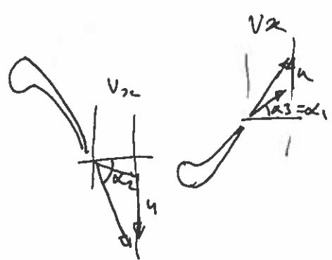
$$\Lambda = \frac{\Delta h_{\text{rotor}}}{\Delta h_{\text{stage}}} = 1 - \frac{\Delta h_{\text{stator}}}{\Delta h_{\text{stage}}}.$$
