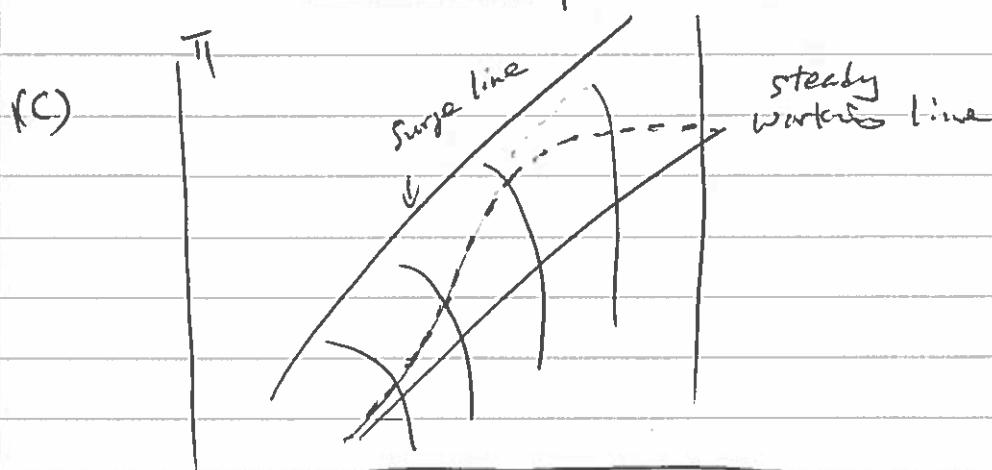
During acceleration turbine power is larger than the compressor power. more fuel is needed to increase  $T_{03}$ . this shall limit mass flow rate through the turbine throats thus shifts the work
