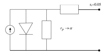
$$r_{o} = \frac{V_{oC}}{I_{sC}} = \frac{0.6}{2.94} = 0.205$$
