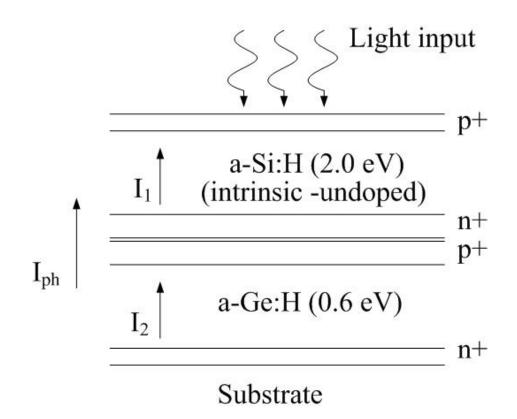
This is equivalent to two cells connected in series. Hence the current condition is  $I_1=I_2=I_{ph}$ .  $I_1$  and  $I_2$  are generated in the two different absorber layers from different parts of the solar spectrum, where the energy flux (photon flux) is different for different wavelengths
