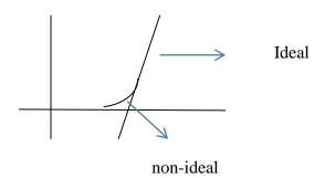
When operating as a solar cell the softer turn-on is seen as a loss of  $V_{OC}$ .
